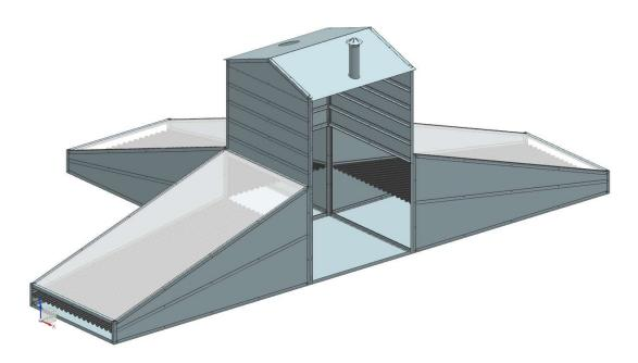
Step 24) Attach the roof assembly and the solar dryer at the locations indicated (repeat on the opposite side).
