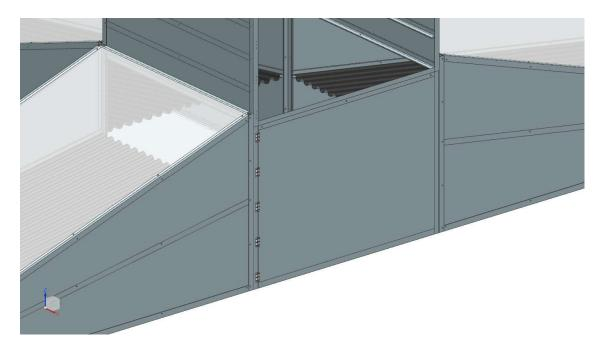
Step 26) Secure Parts 27 and 28 to the upper cabinet and secure the upper cabinet door (Part 29) as shown below.
