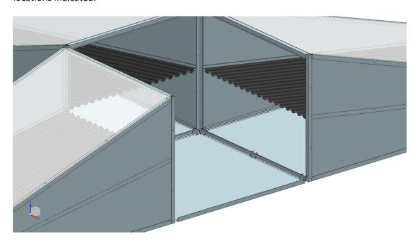
Step 13) Align the assembly in Step 11 with the solar dryer assembly. Connect at the locations indicated and repeat for 15a, 15b, 15c and 15d.
