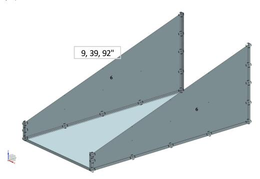
Step 4) Secure Parts 7 with the previous assembly at the locations circled. Note: Some of the previous screw locations in the previous step will be reused.
