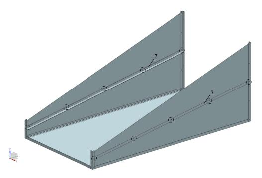
Step 5) Rest Part 8 on the assembly in Step 4 such that it rests on Part 5.
