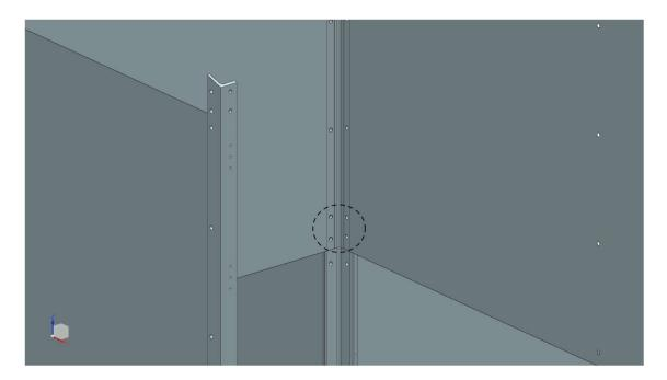
Step 18) Secure Part 19 (the 15 shelf pieces) as shown below. There are three screw locations for each shelf. Some screws may have to be unscrewed and reattached where the upper cabinet connects with the lower cabinet and solar collectors.
