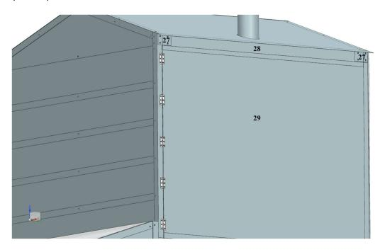
Step 27) Secure magnetic tape along Parts 28, 14 and the faces of Parts 3a, 15d and 17d that the doors of the cabinets overlap on.
