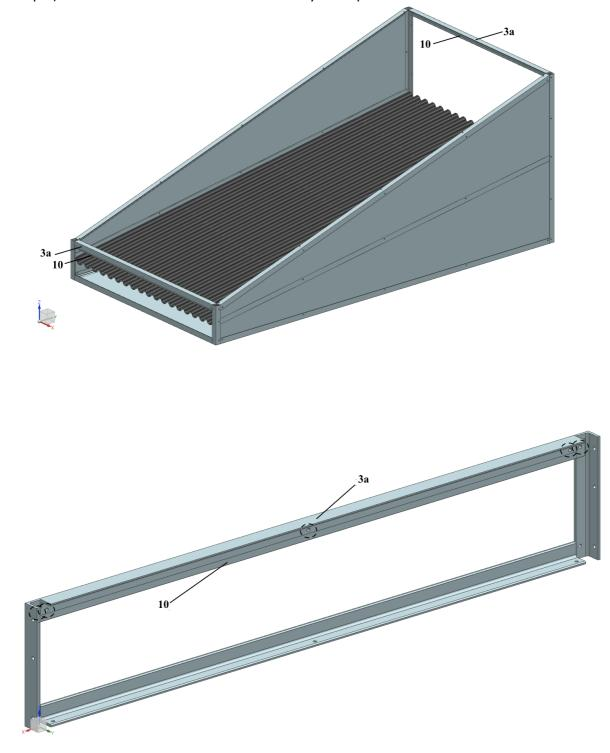
Step 7) Secure Parts 10 and 11 to the assembly in Step 6 at the locations circled.
