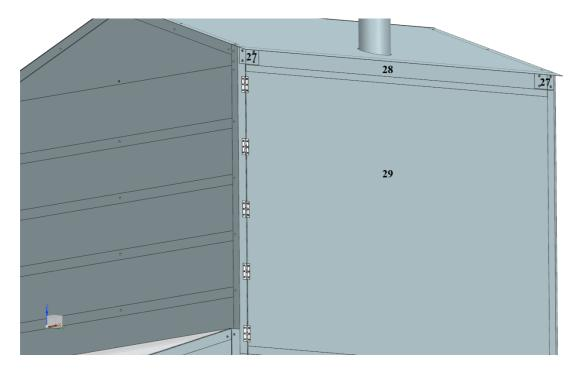
Step 27) Secure magnetic tape along Parts 28, 14 and the faces of Parts 3a, 15d and 17d that the doors of the cabinets overlap on.
