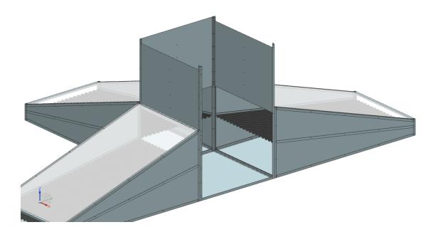
Step 17) Secure the parts in Step 16 together at the locations indicated (repeat at identical locations on 17a, 17b, 17c and 17d). Note: some bolts may need to be unscrewed and rescrewed in order to secure the parts.
