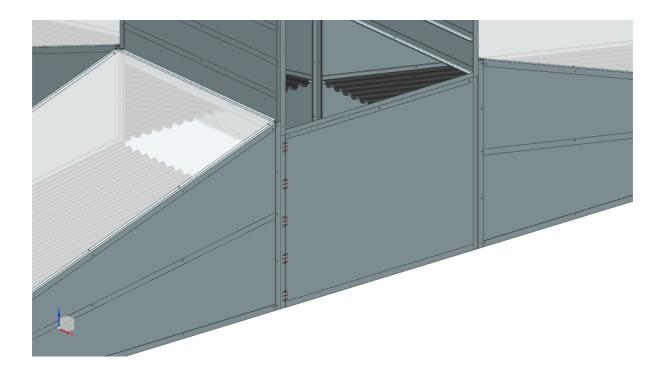
Step 26) Secure Parts 27 and 28 to the upper cabinet and secure the upper cabinet door (Part 29) as shown below.
