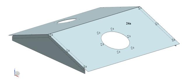
IF USING THE CHIMNEY: Use only one Part 24b and secure it to the assembly in Step 20. Weld the chimney to Part 24b (where the opening is and stick the chimney about 2-3 inches below the surface of Part 24b) once it is assembled after the next step.
