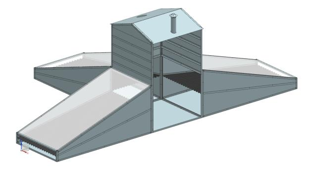
Step 24) Attach the roof assembly and the solar dryer at the locations indicated (repeat on the opposite side).
