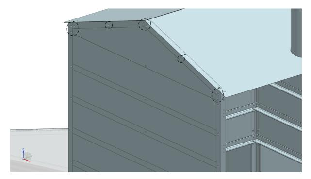
Step 25) Attach the lower cabinet door to the solar dryer with the hinges.
