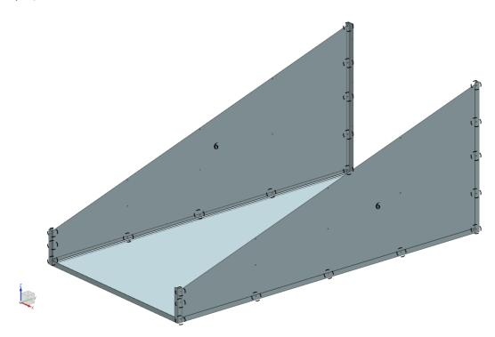
Step 3) Secure Parts 6 to Parts 4 and 5 at the locations circled
