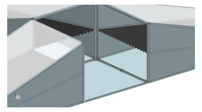
Step 13) Align the assembly in Step 11 with the solar dryer assembly. Connect at the locations indicated and repeat for 15a, 15b, 15c and 15d.
